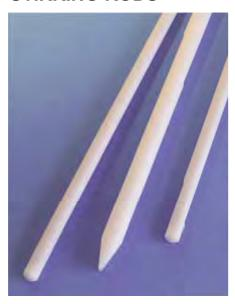
Stirring Rods are available in two versions. Pure PTFE solid rod with tapered end and pure PTFE with mild steel core. The version with steel core can be bent into a permanent shape. Inert and will not scratch, use up to 280°C.
