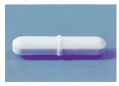
Pivot Ring Stirrer Bars are for use in containers with bases that are slightly curved or uneven - the pivot enables the stirrer to adopt the optimum position for stirring.
